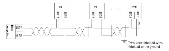
It is recommended to add a matching resistor between A and B of the end meter,and the resistance range is 120  $\Omega$  -10K  $\Omega$  .
