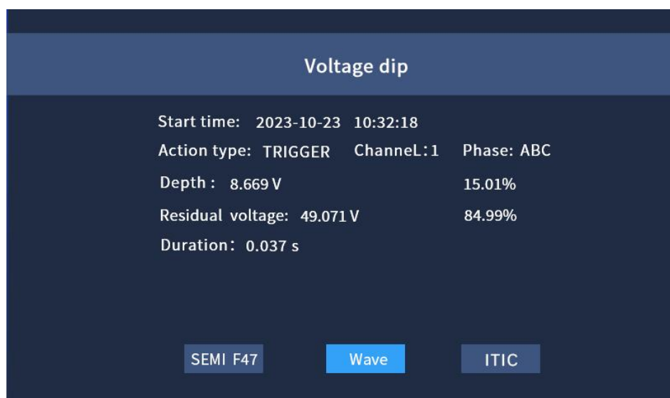
Fig. 4.22(a) Voltage dip
